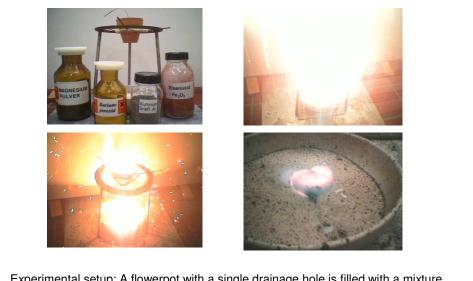
Experimental setup: A flowerpot with a single drainage hole is filled with a mixture of iron oxide ( $Fe_2O_3$ ) and coarsely ground aluminum (reaction mixture: Thermit® mixture). This is covered with a mixture of magnesium and barium peroxide ( $BaO_2$ ) (ignition mixture). A strip of magnesium serves as a wick. A porcelain dish filled with sand is placed underneath.
